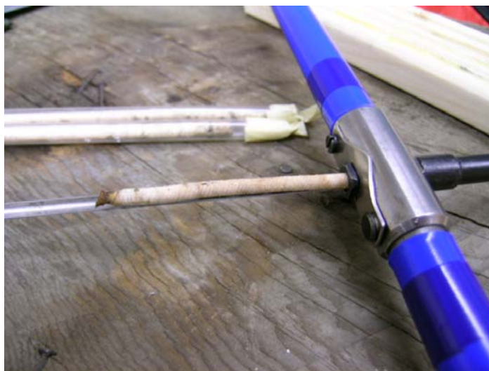
Figure 2: Sample extracted with an increment borer.
