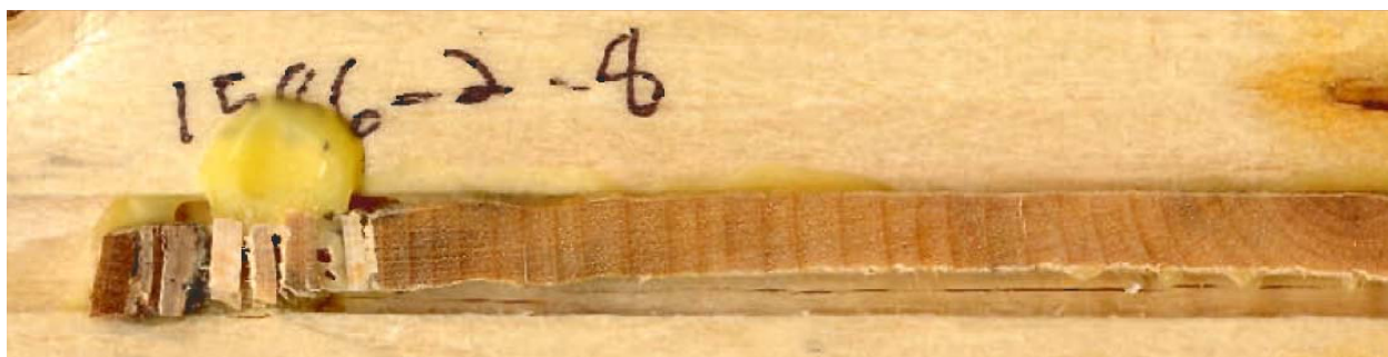
Figure 1. An example (4-08-1586-2-8a) of a core which was too broken up at the beginning to be properly mounted and measured.
