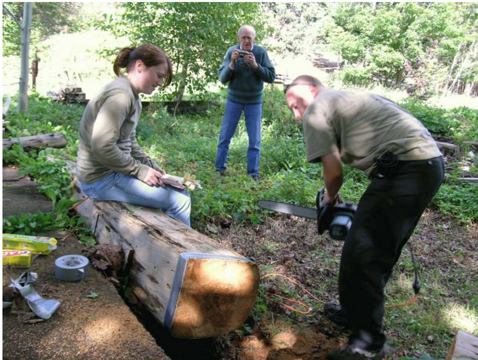
Figure 3 - A sample being taken of one of the remaining barn beams. The footprint of the barn was clearly evident and some of the original structure remained sound enough to sample.
