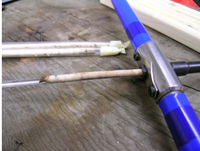
Figure 2: A core being removed from an increment borer. Note that the diameter of the core is about the size of a pencil (4.3 mm).
