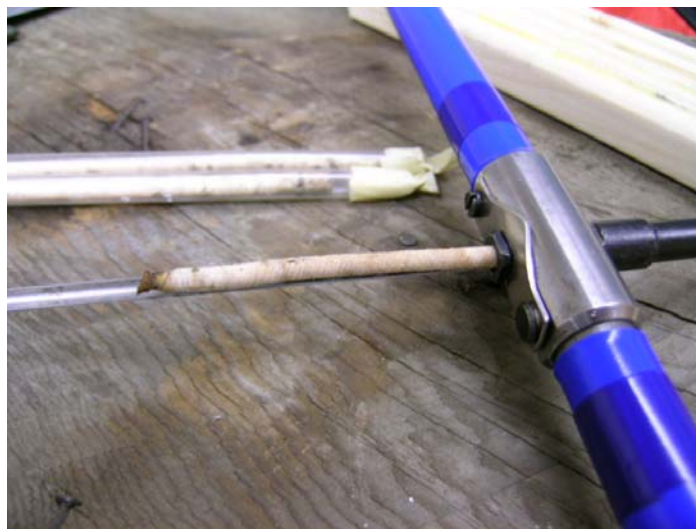
Figure 2: Sample extracted with an increment borer.
