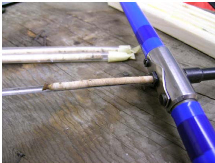
Figure 2: Sample extracted with an increment borer.
