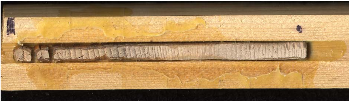
Figure 2 – Image of mounted core (07A003) that has been prepared for measuring.
